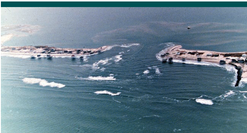
Figure 21. The Westhampton barrier breached during the December 1992 northeast storm forming Little Pike's Inlet in Moriches Bay. (Photo: First Coastal Corp)
