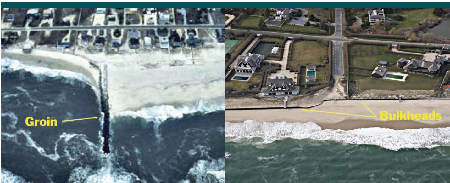
Figure 22. The most commonly used erosion control structures on the south shore are shore perpendicular structures like the groyne on left and shore parallel structures like the bulkheads on right. (Bulkhead photo: First Coastal Corp)
