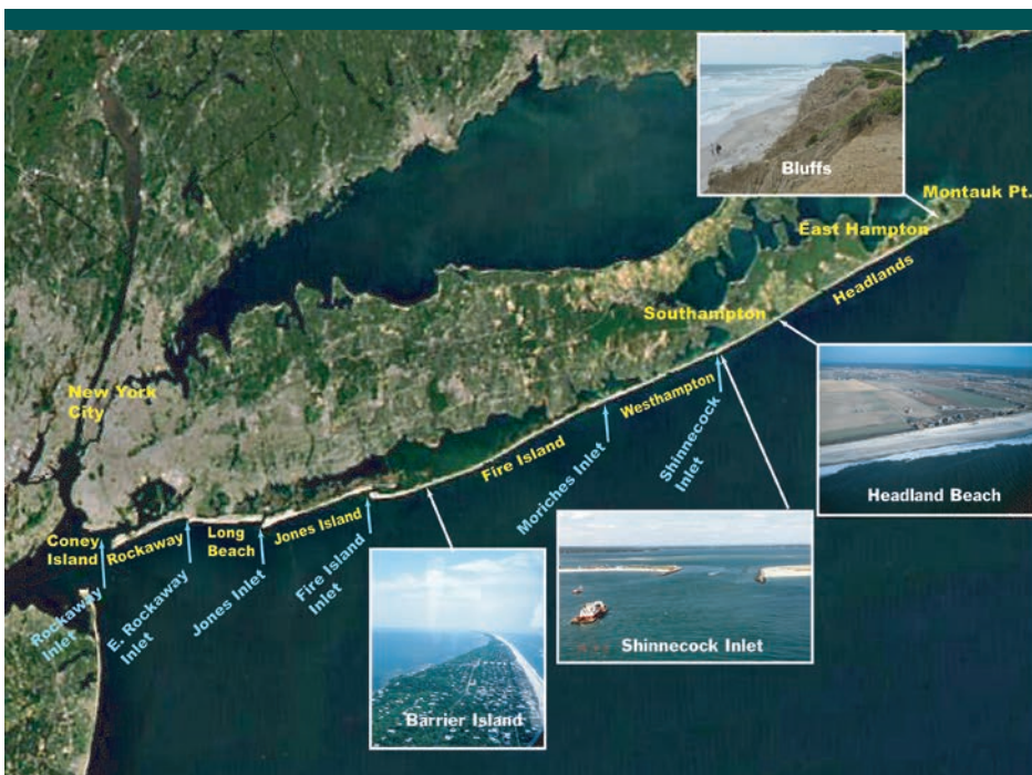
Figure 1. Long Island's south shore includes a variety of different shoreline types including an extensive barrier system with islands separated by tidal inlets in the west and a headlands section with high glacial bluffs in the east. (Satellite photo: NASA Visible Earth http://visibleearth.nasa.gov/ )
