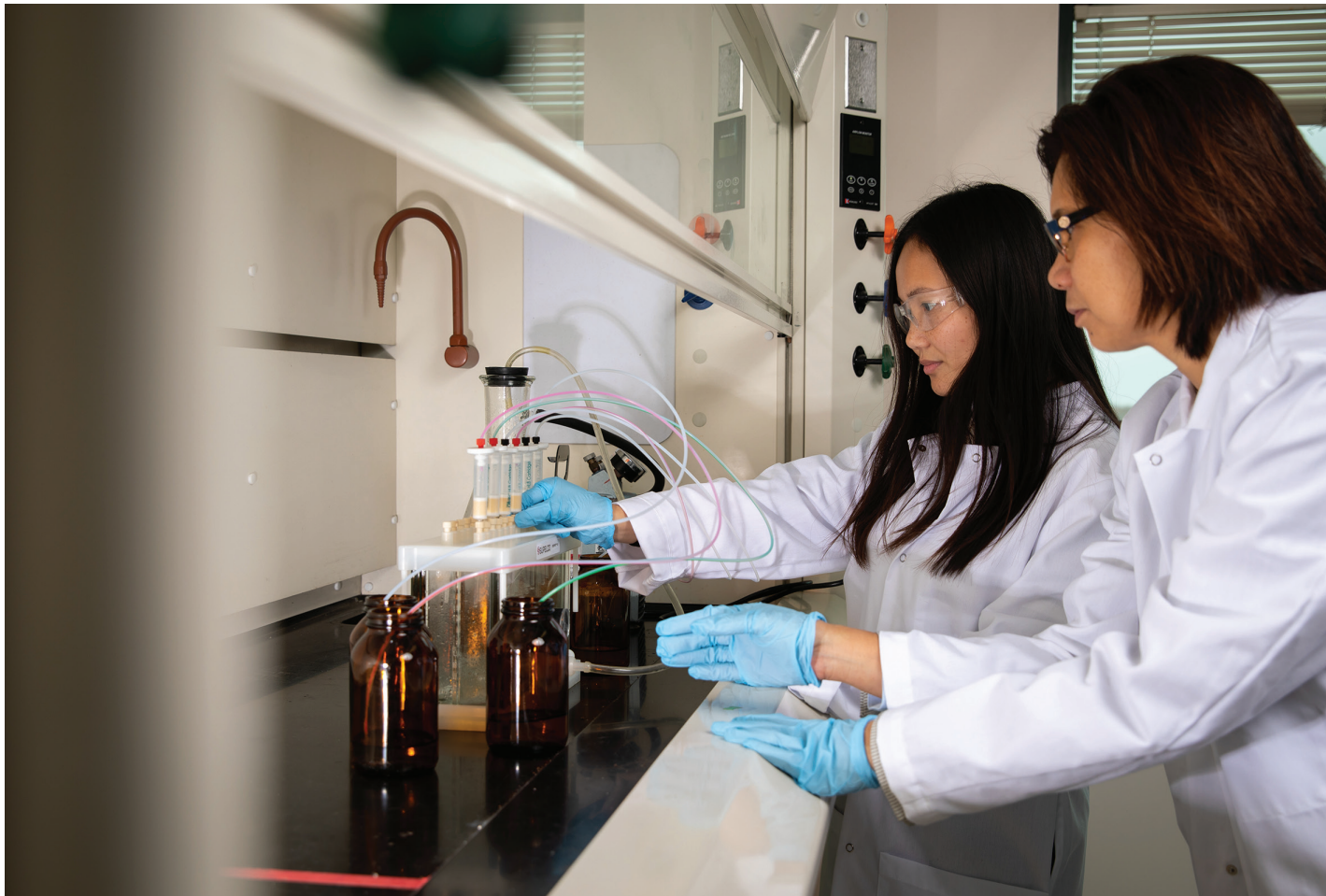
UB chemistry professor Diana Aga (right) and UB chemistry PhD candidate Luisa Angeles in the lab. To study pharmaceuticals in wastewater, they use the system pictured to isolate chemical compounds from the wastewater. Image credit: Meredith Forrest Kulwicki
